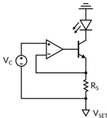
A control loop adjusts the voltage across the transistor  $V_T$  to keep the voltage across the sense resistor  $V_{R_S}$  equal to the control voltage  $V_C$ . The laser current  $I_L$  is then equal to  $V_C/R_S$  ( $R_S = 5\ \Omega$  for the QCL100-A-500)
