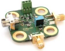
Koheron PD200T is an InGaAs photodetector with a dual TTL-analog output. The analog output has a gain of 500 V/A and a 200 MHz bandwidth. The TTL output has 2.5 ns propagation delay, 1.3 ns rise time and 0.7 ns fall time. Trigger threshold can be adjusted with a precision trimmer.
