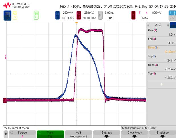
Propagation delay between the analog and the TTL output is about 2.5 ns. TTL rise and fall times (10 to 90 %) are 1.3 ns and 0.7 ns, respectively.
