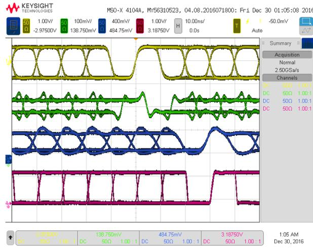
The 25 ns delay between the **laser modulation** (in orange) and the **PD200T analog output** (in blue) corresponds to the 5 m fiber between the laser and the PD200T.
