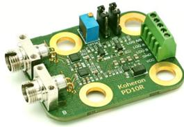
Koheron PD10R is a dual logarithmic photodetector for general purpose optical power measurements. In addition to two analog outputs  $\log(A)$  and  $\log(B)$ , the PD10R gives the log-ratio  $\log(A/B)$  with an adjustable offset and two gain settings (x1 and x10). The PD10R provides a fully-analog solution for direct absorption measurement in spectroscopy setups.
